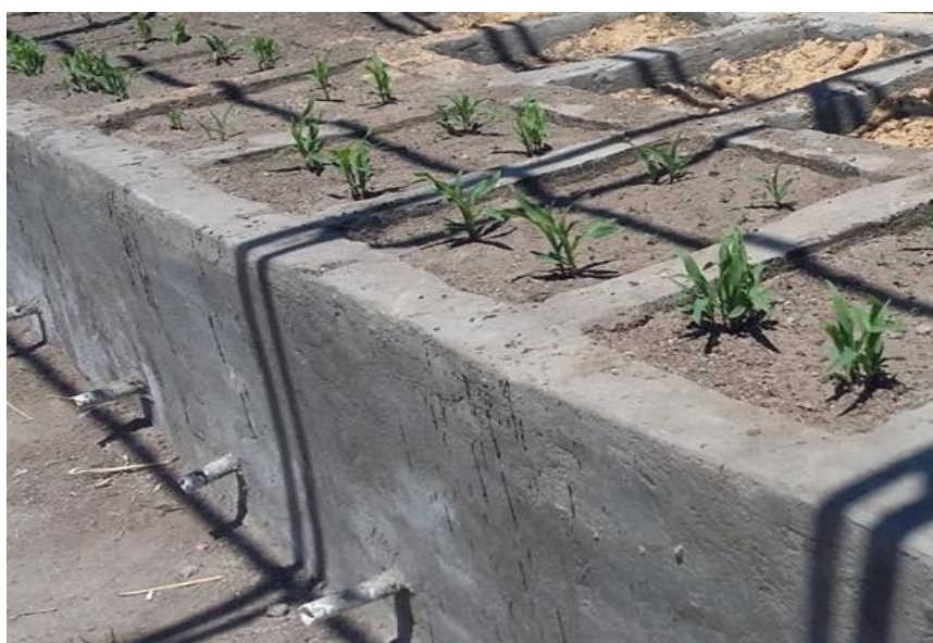
Figure 1. Layout of field lysimeter experiment (60x 60 x 75cm)
