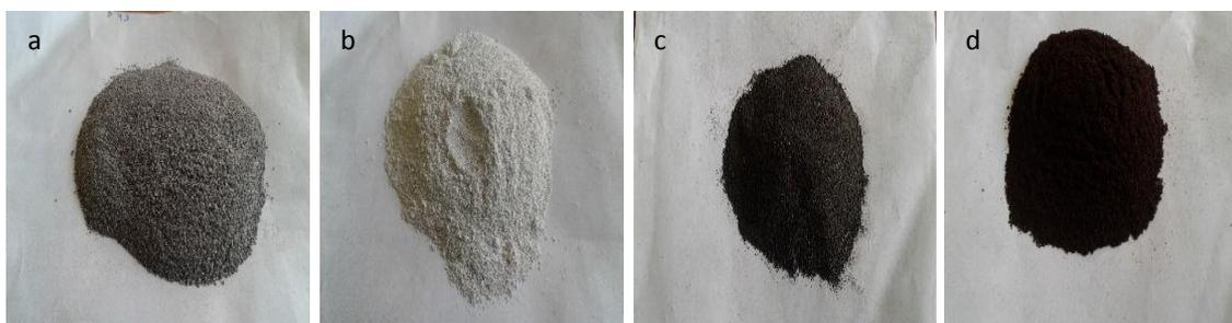
**Fig. 1. Images of calcinated bone-ash (BA) and pyrolyzed bone-char (BC) produced at 600 and 700 °C: (a) BA-600; (b) BA-700; (c) BC-600; and (d) BC-700, respectively.**
