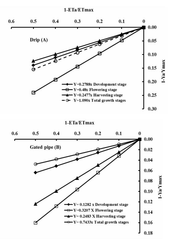
Fig.2. The relationships between the relative tomato fruit yield reduction and relative evapotranspiration under drip (A) and gated pipe (B) irrigation systems
